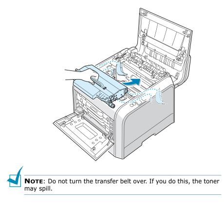
**13** Slide the transfer belt down into the printer and press it firmly into place.
